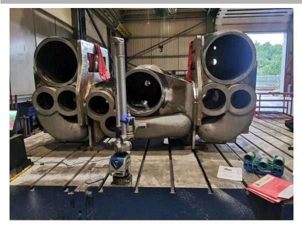
Welcome to the 91<sup>st</sup> edition of *The Mikado Messenger*, bringing you the latest update from No. 2007 *Prince of Wales*. This month we focus on the cylinder block assembly, which is entering the latter stages of fabrication at Howco in Irvine.
