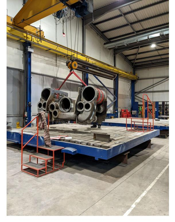
Picture of the unit being maneuvered off the surface table after being welded such that it can be lifted. The monobloc is seen undergoing its pre final weld inspection.
